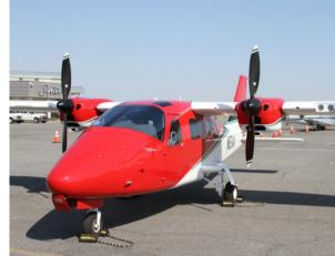
Flexible and economical, Tecnam P2006T is a twin-engine four-seat aircraft with fully retractable landing gear with a class of its own. The superior high-wing configuration offers stability, superior cabin visibility and easy access for passengers and luggage. Tecnam has used its extensive experience with aluminum airframes to create in the Tecnam P2006 a robust yet very light airframe, resulting in an outstanding payload-to-total weight ratio.
